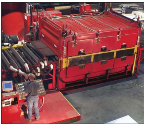
The SCS Sheet Line employs engineered abrasive brushing rolls and ordinary water in a simple, compact, low cost process.
